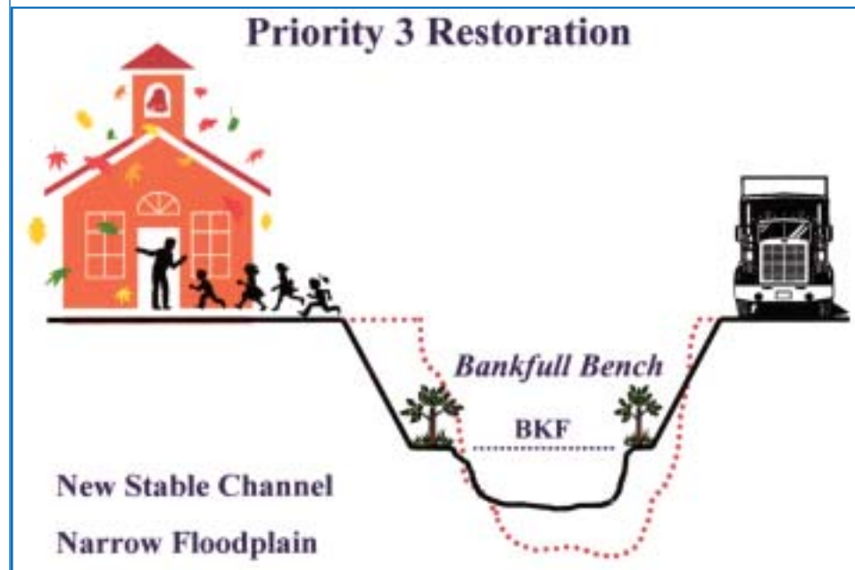
Figure 5.4 Cross section of a Priority 3 restoration project
